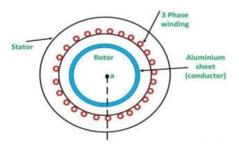
The basic design and construction of a linear induction motor is similar to a three phase induction motor, although it does not look like a conventional induction motor. If we cut the stator of a polyphase induction motor and lay on a flat surface, it forms the primary of the linear induction motor system. Similarly, after cutting the rotor of the induction motor and making it flat, we get the secondary of the system.
