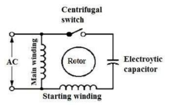
• In single phase induction motor main winding is designed for low resistance & starting winding for high resistance. Phase difference in both winding is produced by connecting capacitor in series with starting winding. Direction of rotation of single phase induction motor depends upon the instantaneous polarities of main winding flux & starting winding flux. So direction of rotation can be changed by reversing the polarity of either main or starting winding as shown in figure.
