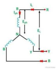
In star connection line voltage is root 3 times of phase voltage.
