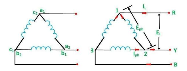
To obtain the **delta connections**,  $a_2$  is connected with  $b_1$ ,  $b_2$  is connected with  $c_1$  and  $c_2$  is connected with  $a_1$  as shown in the above figure. The three conductors R, Y and B are running from the three junctions known as **Line Conductors**.
