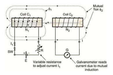
VII Actual Circuit diagram used in laboratory with equipment Specifications:
